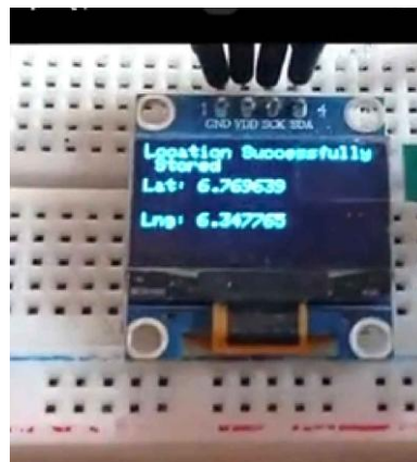
Figure 2: OLED confirming stored reference location showing “Location Successfully Stored” with exact coordinates
