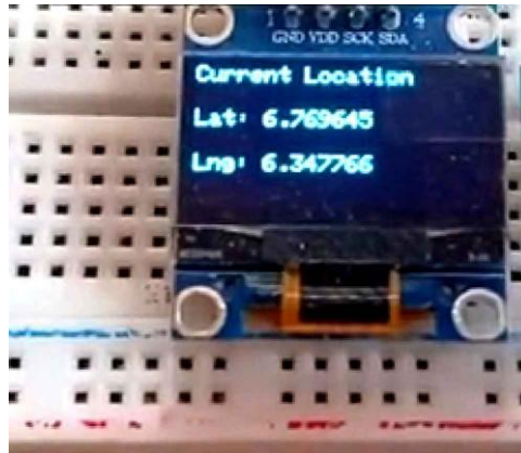
Figure 1: OLED display showing current GPS location showing “Current Location” with clear Lat: 6.769645 Lng: 6.347766
