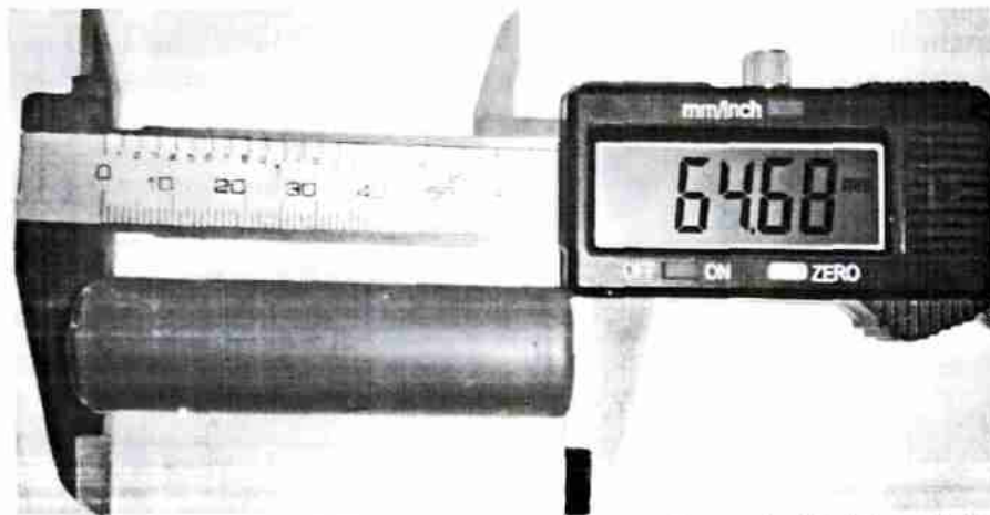
Figure 1: a 2600mAh 18650 Li-ion battery, measuring only 65.57mm in length
