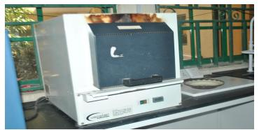
Plate 1: The Muffle Furnace used for the determination of Ash Content
