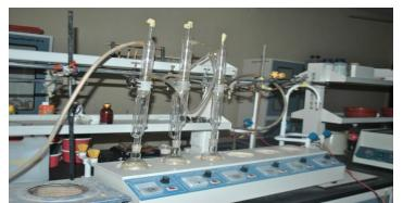
Plate 2: Soxhlet apparatus for fat determination (DHG-9023A, England)
