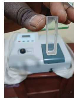
Plate 3. Cuvette that hold honey sample in the Ultraviolet-Visible Spectroscopy (Spectrophotometer) to detect presence of phytochemicals in qualitative screening.
