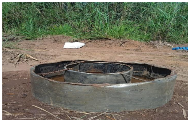
Plate 1: Double ring infiltrometer in the field
