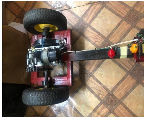
Fig. 5 Mechanical and electrical components of the automatic braking system
