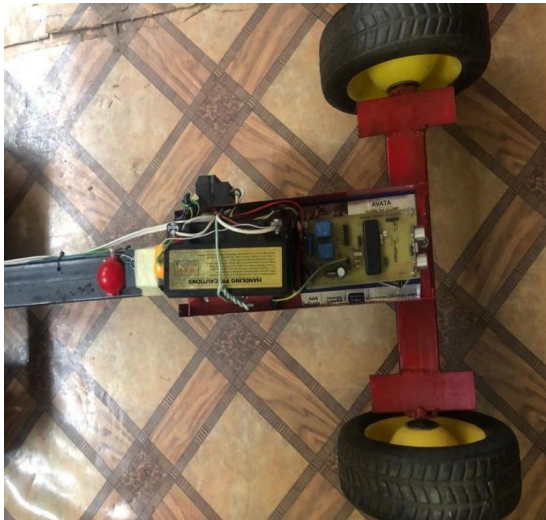
Fig. 5 Mechanical and electrical components of the automatic braking system
