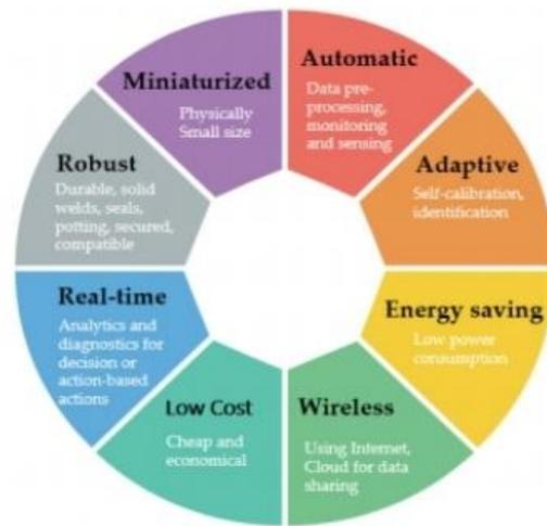
**Fig. 2:** Main characteristics of intelligent sensors (Pech et al., 2021)
