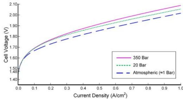
Figure 6. The impact of pressure on the performance of the PEM electrolyser at 300 K. The stack's performance depends heavily on temperature and pressure, which also affect the thermo-neutral voltage. The model was tested at atmospheric, 20, and 350 bars. Above 1.48 V, electrolysis begins, with similar trends observed in graph paths as current density rises.
