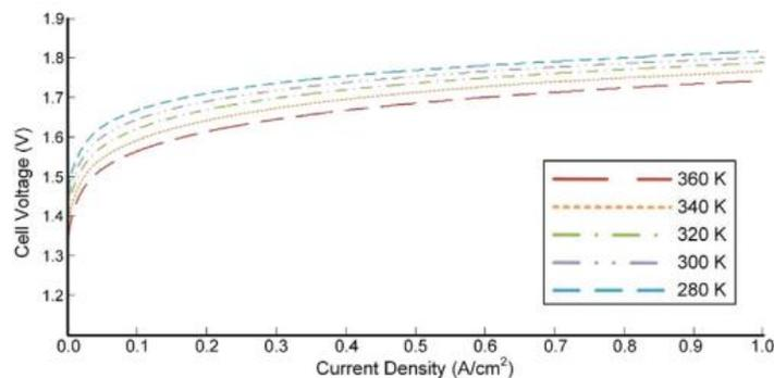
Figure 7. The impact of temperature on the performance of the PEM electrolyser stack under standard atmospheric pressure.
