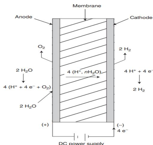
Figure 2. A PEM water electrolysis cell and its corresponding half-cell reactions. (Kritharas & Watson, 2010)
