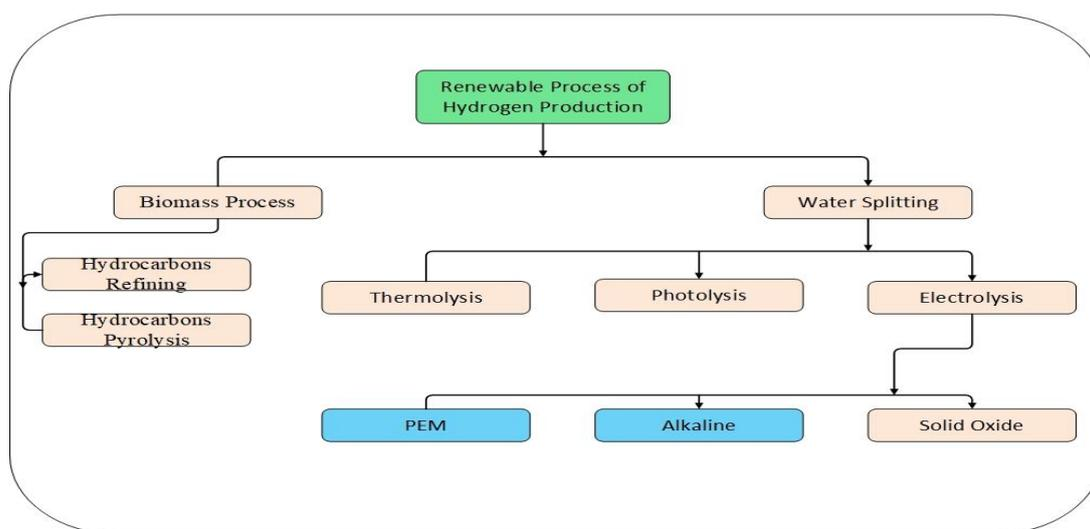
Figure 1. Hydrogen production methods
