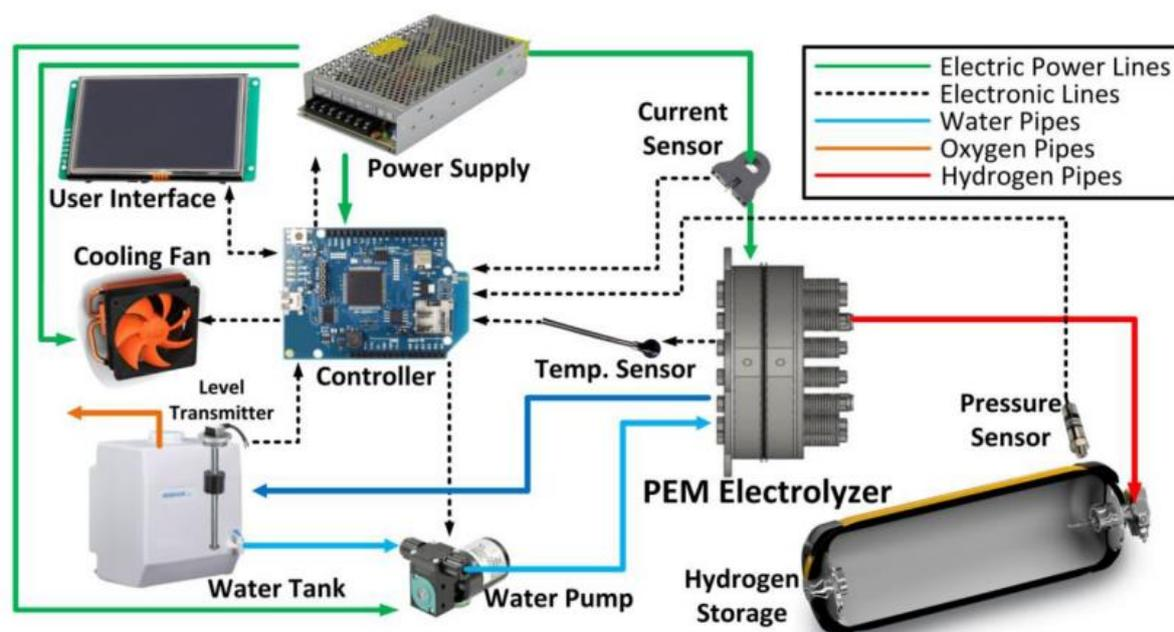
Figure 4. The PEM electrolyser system utilised for the development of the dynamic model by Yigit & Selamet, (2016).
