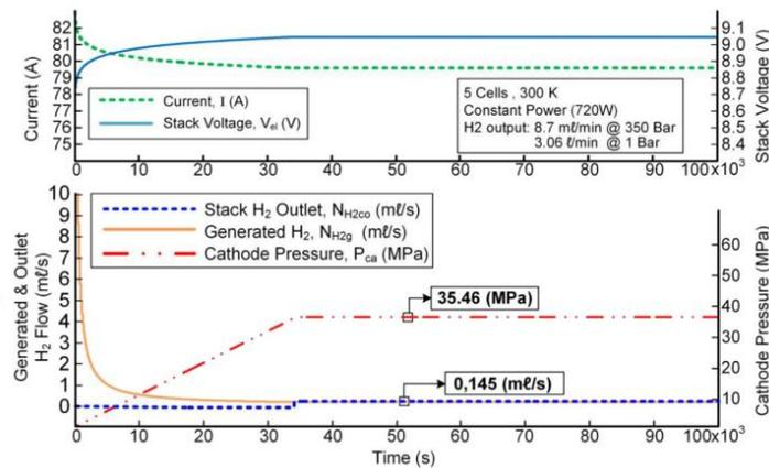
Figure 8. The model results pertain to a fixed power consumption scenario for compressing the produced gas to 350 bars. The power utilised by the stack is capped at 720 Watts.
