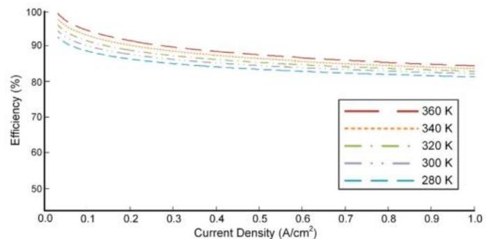
Figure 9. The impact of current density on the efficiency of the PEM electrolyser at various temperatures under standard atmospheric pressure.
