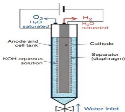
Figure 3. A Monopolar alkaline water electrolysis cell.
