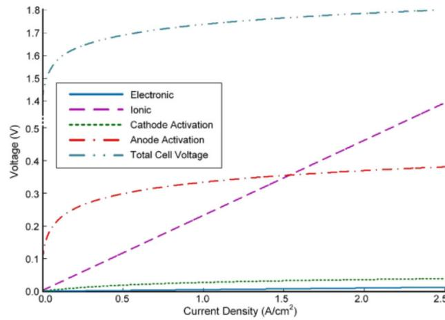
Figure 5. The impact of current density on over potentials and the performance of the PEM electrolyser stack under standard conditions of atmospheric pressure and 300 K.
