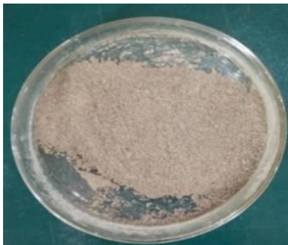
Figure 4: Zinc-Graphene Nano-composite after synthesis
