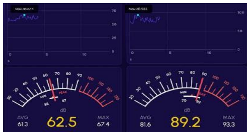
Figure 2: The Mower's Sound Level at 0.7 m (Left) and 0.1 m (Right) from Exhaust Port
