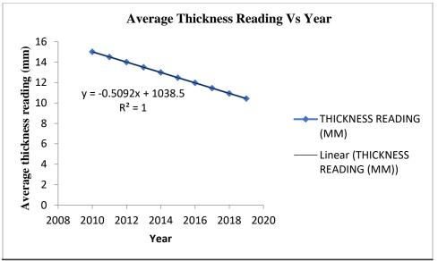
Figure 1. Plot of average Pipe Wall Thickness Vs. Year
