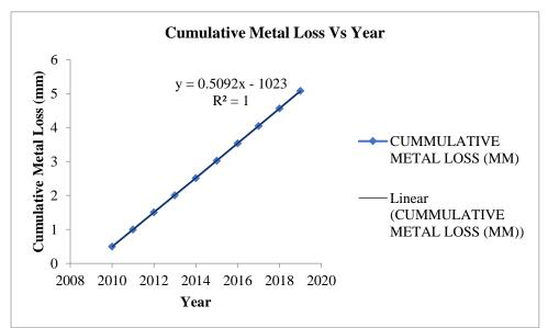
Figure 3.3: Plot of Cumulative Metal Loss Vs. Year
