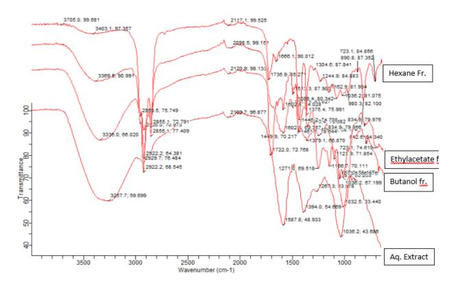
Figure 1: superimposed FTIR Spectra of the aqueous ethanol leaf Extract and fractions of *P. senegalensis*
