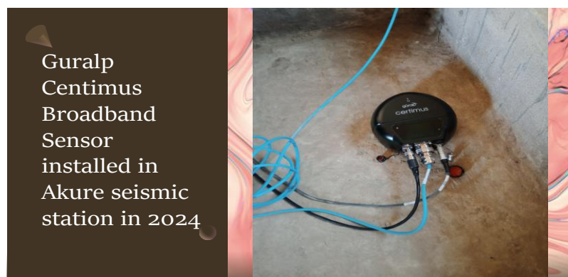
Fig. 1.5: Guralp Centimus Sensor installed in Akure
