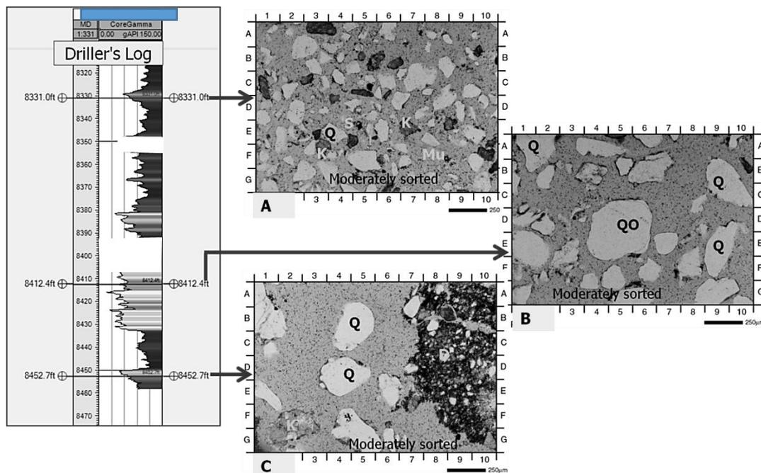
**Fig.4: (A – C): Thin-section photomicrograph showing effects of compaction and cementation on framework minerals (D = Detrital Clay, K = K-feldspar, Q = Quartz, S = siderite Overgrowth, QO = Quartz Overgrowth, Mu = Muscovite)**
