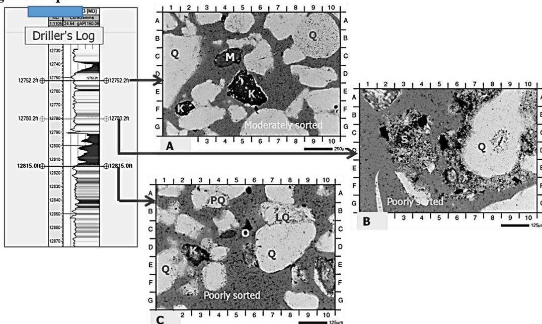
**Fig.6: (A – C): Thin-section photomicrograph showing effects of compaction & cementation on framework minerals (Q-Sand; Zebra-2ST3 Well) (Q = Quartz, PQ = Polycrystalline Quartz, LQ = Leached Quartz, M = Mudstone clasts, K = K-feldspar, S = Siderite patches, O = Authigenic Opaque)**
