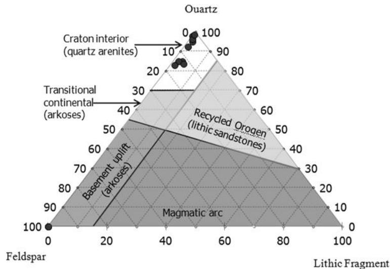
**Fig.7: Quartz-Feldspar-Lithic Fragment (QFL) Ternary plots showing Zebra reservoir sandstone composition and their tectonic setting (modified after Dickinson *et al.*, 1983)**
