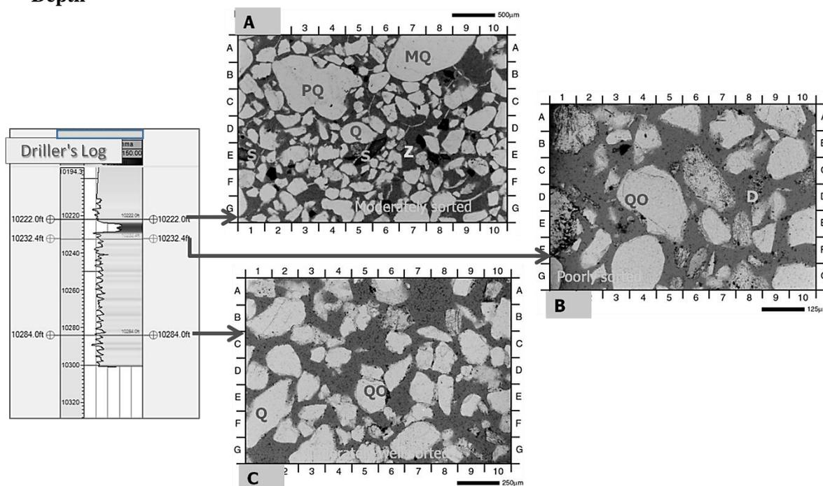
Fig.5: (A – C): Thin-section photomicrograph showing effects of compaction & cementation on framework minerals (R-Sand; Zebra-3 Well) (Q = Quartz, QO = Quartz Overgrowth, PQ = Poly Quartz, MQ = Mono Quartz, D = Detrital Clay, K = K-feldspar, Z = Zircon, S = siderite, O = Authigenic Opaque)
