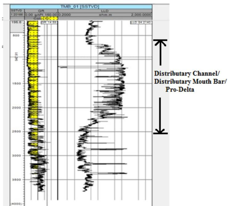
Fig. 6: Identified depositional environments within the subsurface of Tomboy field
