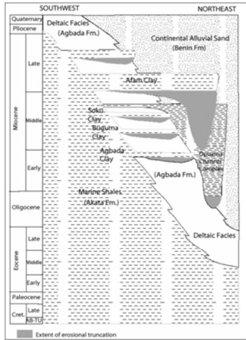
Fig. 2: Stratigraphic column showing the three formations in the Niger Delta [3]
