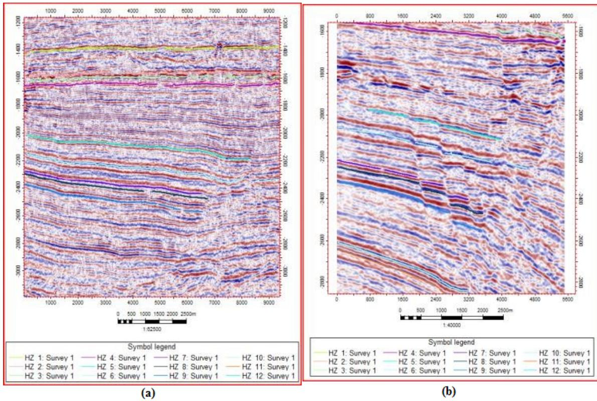
Fig. 8: Mapped Horizon in (a) Seismic crossline (b) Seismic Inline
