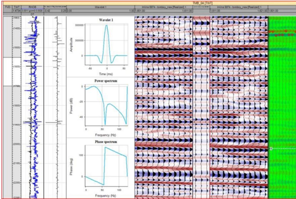
Fig. 7: The synthetic seismogram of the Tomboy field at well 4
