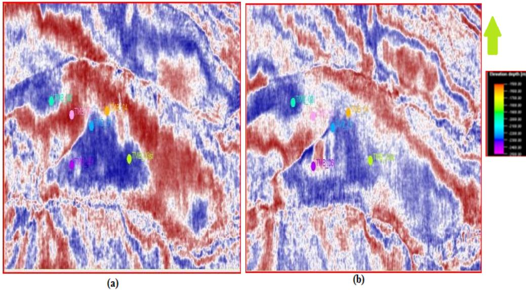
Fig. 9: Time slice at 2372ms and 2649ms: (a) Z slice across Horizon-5 and (b) Z slice across Horizon-6
