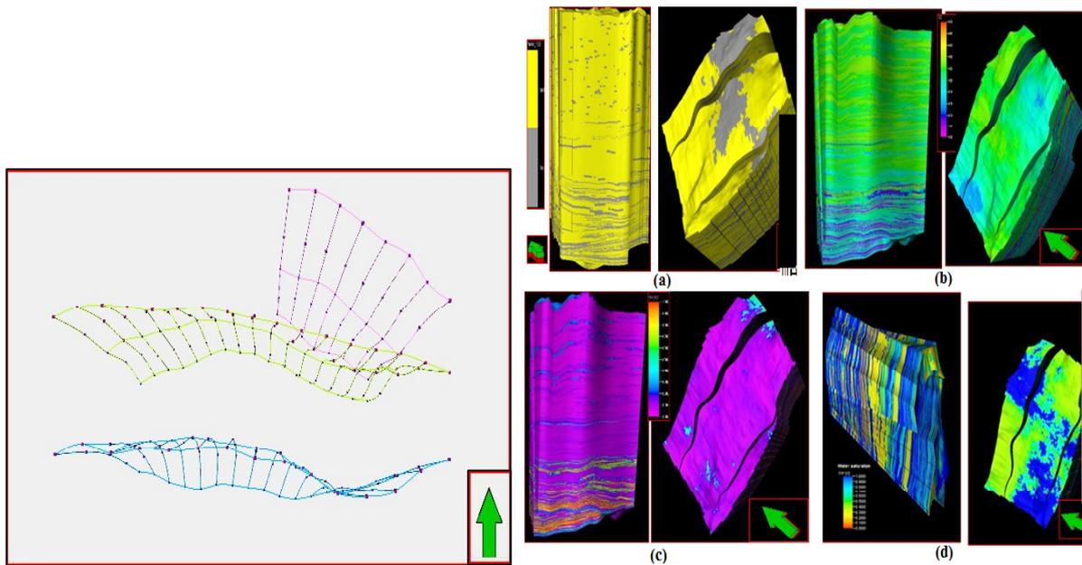
Fig. 12: Fault model of three major identified faults in the area
