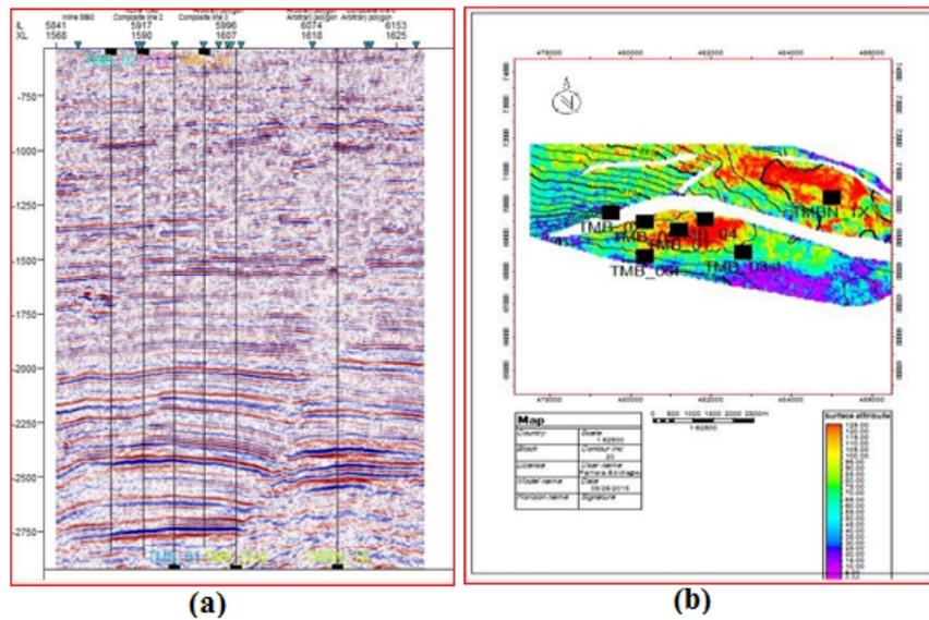
Fig. 16: The proposed wells locations for the new prospect: (a) on a seismic section; (b) in RMS amplitude map
