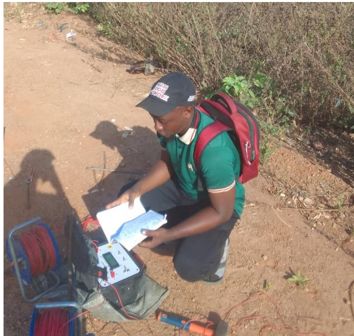
Fig. 3 Researcher and field instruments during VES survey for road failure investigation within the study area.
