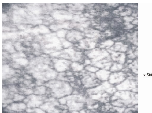
Figure 8: Microstructure of the Weldment
