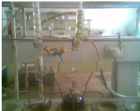
Plate 1: Soxhlet Extraction Apparatus with the extracted oil
