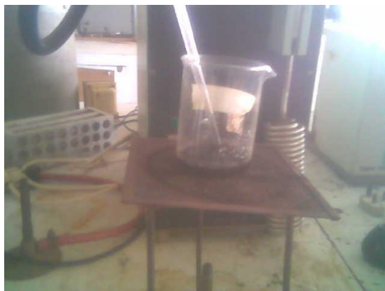
Plate 2: Grease production set-up
