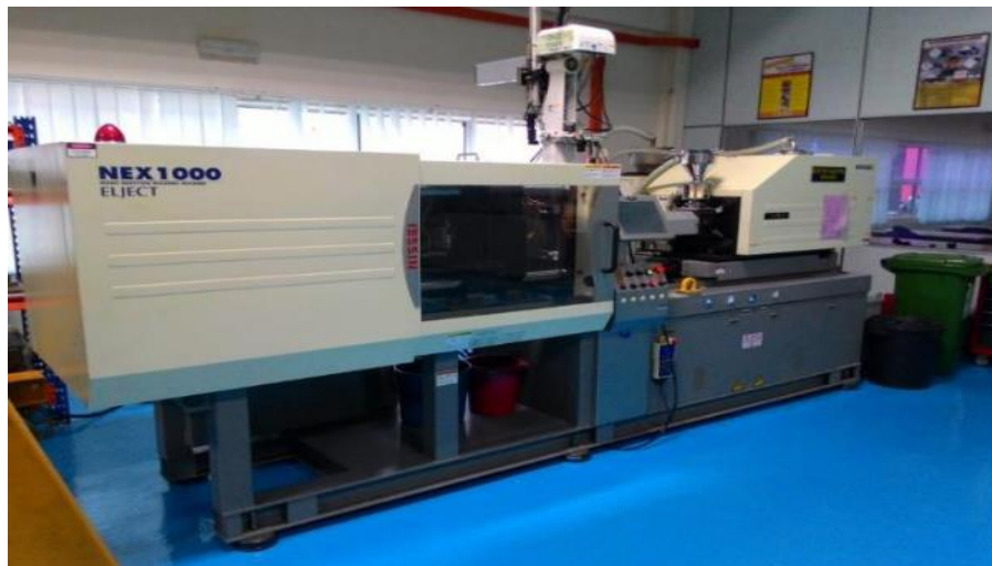
Figure 1: Plastic Injection Moulding Machine (Nissei NEX1000).
