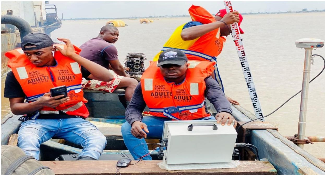
Plate 2: Bathymetric equipment inside survey boat and the crew members the basic principle involves sending an acoustic pulse from the transducer, which travels through the water and reflects off the seafloor. The echo sounder measures the time it takes for the pulse to return, and from this, it calculates the depth.
