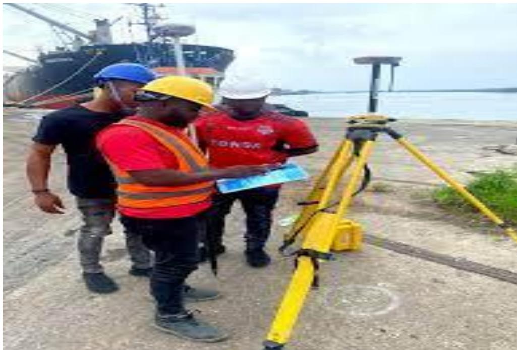
Plate 3: GNSS RTK base station on a control point
