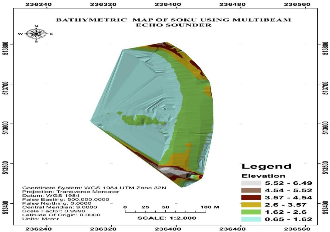
Figure 10a: Aerial view of Bathymetric Map of Soku using Multi-Beam Echo sounder
