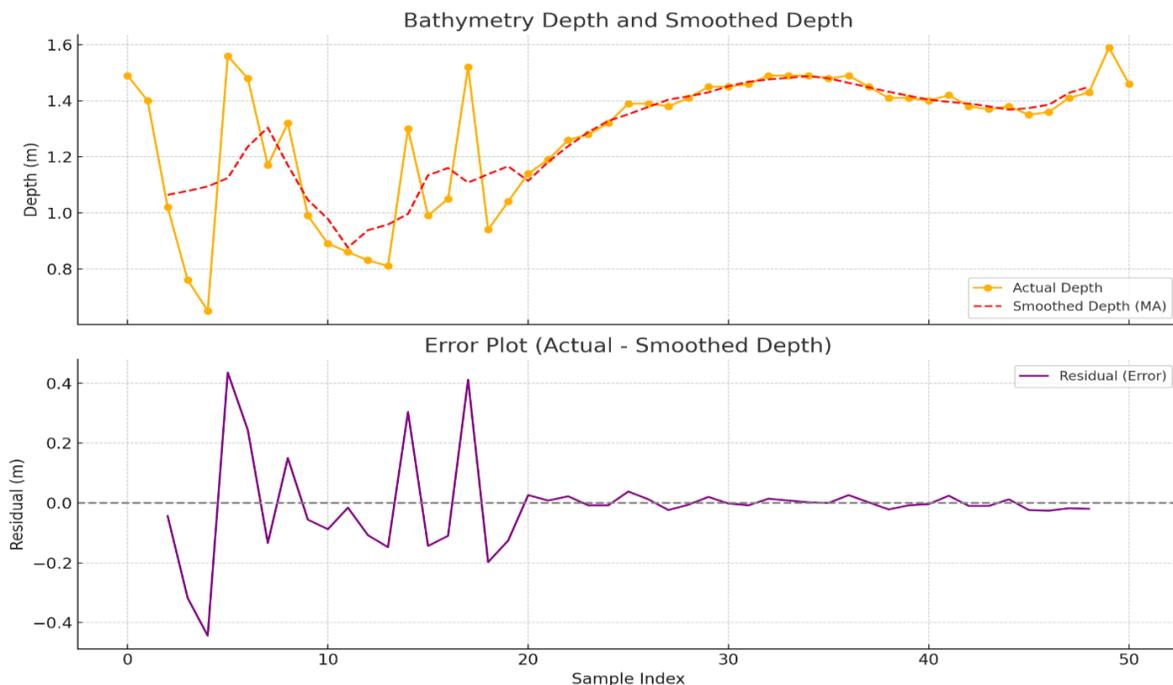
Figure 4: The error plot of the depth
