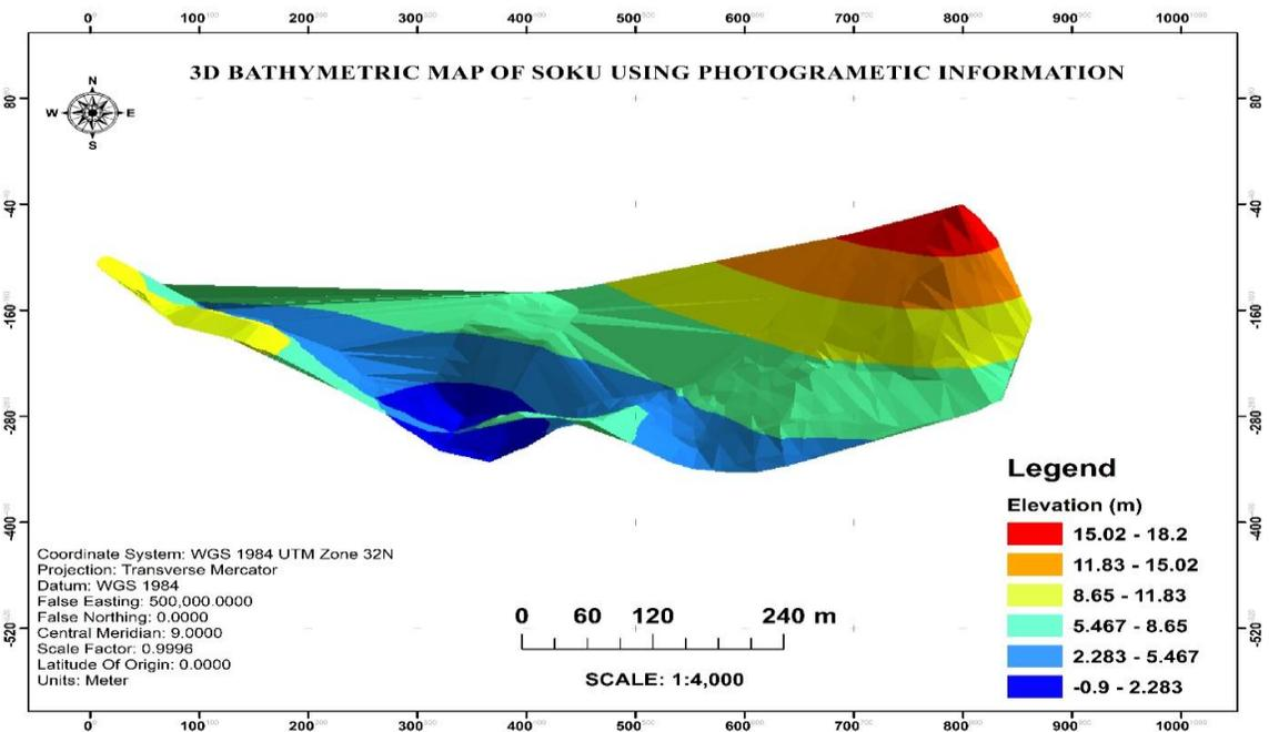
Figure 9b: 3D Bathymetric Map of Soku using Photogrammetric Information.
