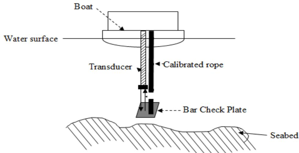
Figure 3: Bar Check Calibration, Source: [11]
