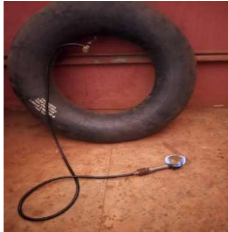
Figure 5: Flame test (gas stored in the tube)
