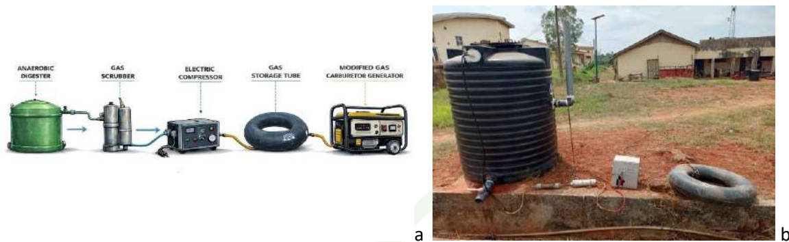
Figures 1(a and b): Biogas Design (A) Design Sketch (B) Pictorial View of The Biogas Digester.
