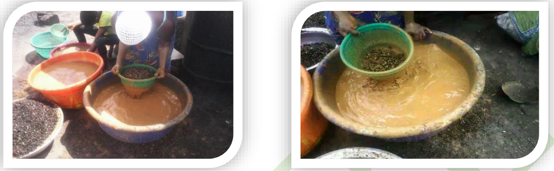
Plate. 1: Traditional method of separating kernel from shell using clay bath method (Local Oil Palm Processing Mill at Ovia North East, Edo State, 2013)
