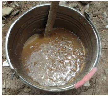
Fig. 2: Mixing feedstock with the starch
