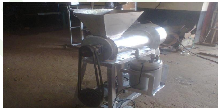
Figure 1: Pictorial view of the improved cassava pelletizer
