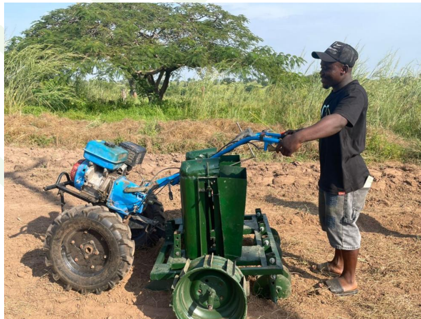
Figure 4: View of the Fabricated Two-Row Irish Potato Planter Hitched to a Power Tiller
