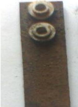
Fig. 3. Coupon immersed in produced water, corr. rate =40mpy.
