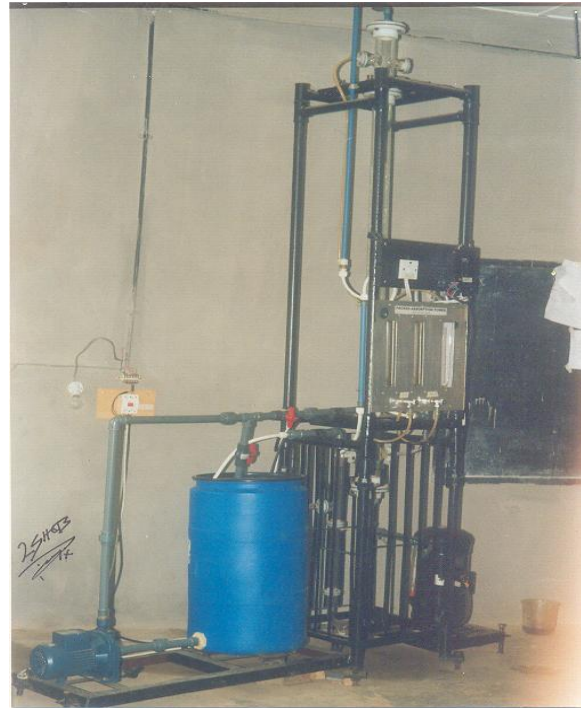
Fig. 2. The photograph of the packed tower absorption apparatus after completion.
