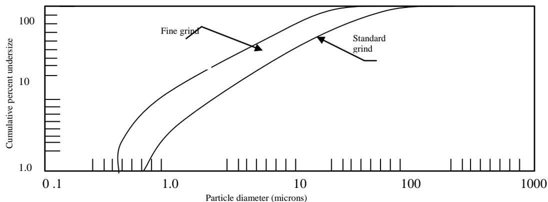
Fig. 4. Particles size distributions for cwfs used in study.
