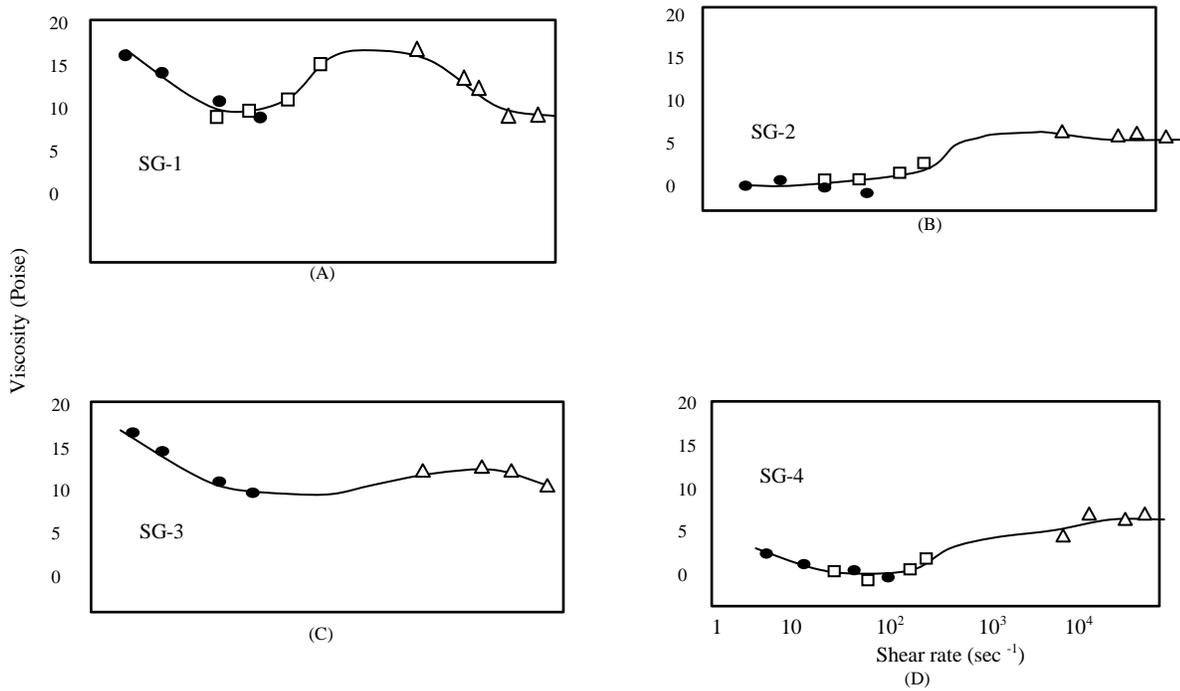
Fig. 6. Rheograms obtained for 70% standard grind cwfs made with four different additive packages.
