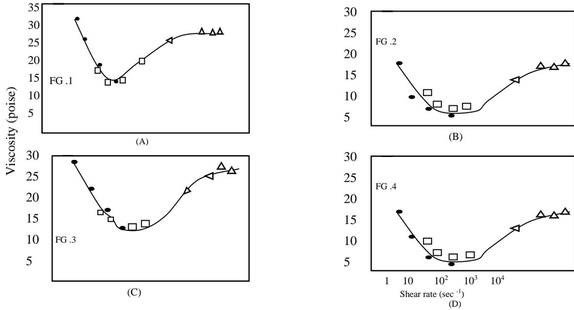
Fig. 5. Rheograms obtained for 70% fine grind CWFs made with four different additive packages.
