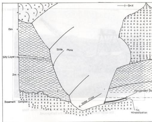
Fig. 2. Vertical section of a paddock in Sabon Gidan Kanar tin mine. Notice the mineralized zone.
