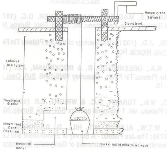
Fig. 5. Vertical section of a lotto mine.
