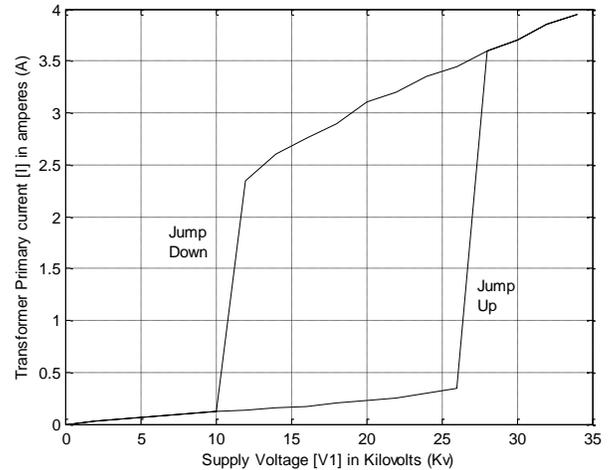
Figure 7 Graph of Primary induced current versus supply voltage at no-load during unsymmetrical switching of the transformer
