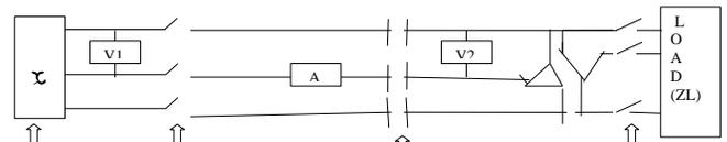
3Ø power Primary Switch Capacitors Secondary Source Switch
