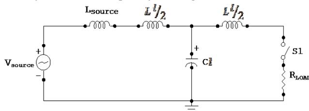
Figure 1.0: equivalent circuit of 1-phase conductor for the calculation of Ferranti rise
