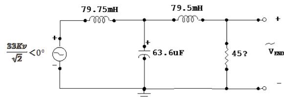
Figure 2: Ferranti rise in cable under load condition
