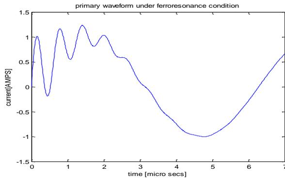
**Fig11: distortion of primary waveform due to ferroresonance**
