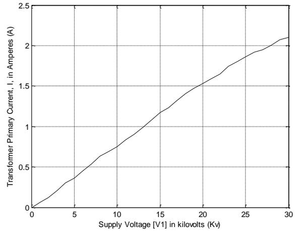
Figure 9: Graph of Primary induced current versus supply voltages when the transformer is on-load.
