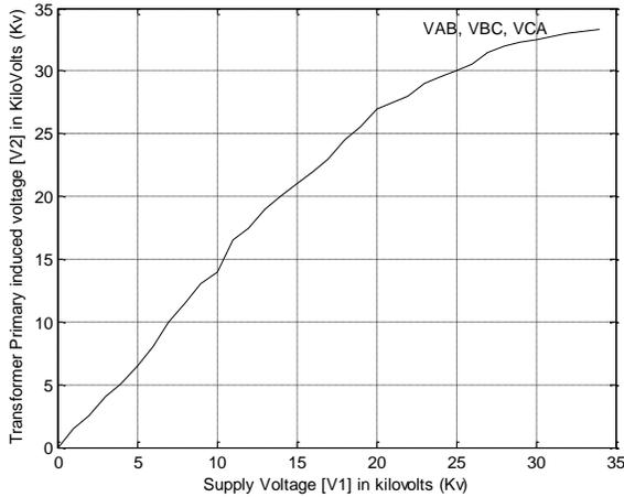
Figure 8: Graph of primary induced voltages against supply voltages when the transformer is on-load
