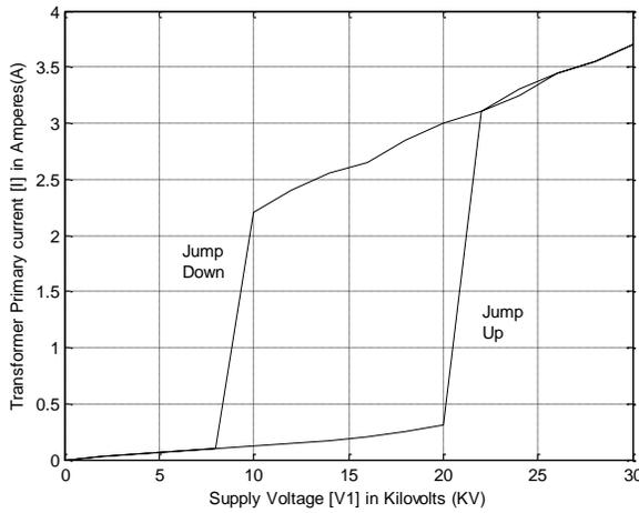
Figure 5.0: Graph of Primary induced current versus supply voltage at no-load.
