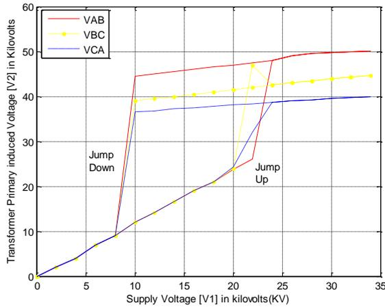
Figure 4.0: Graph of primary terminal voltage against supply voltage at no load
