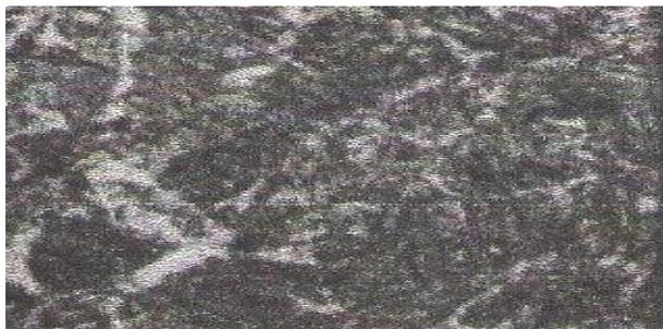
Fig. 2. Weld Microstructure made from the vertical position.
