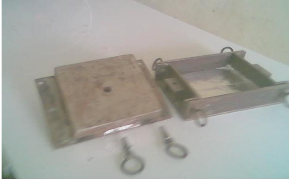
Fig. 3. A two-part mould (cope and drag).
