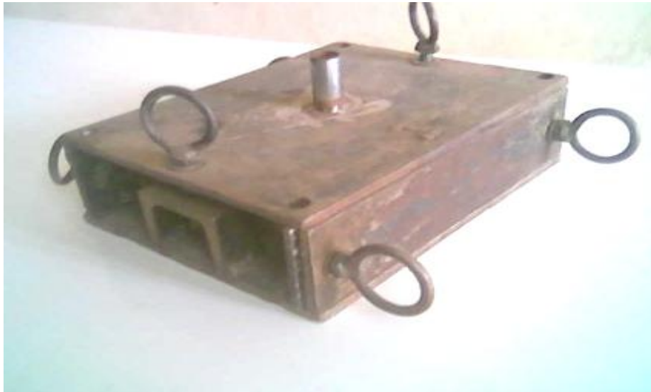
Fig. 4. A-two part mould (assembled).
