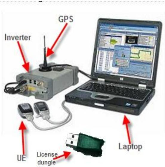
Figure 2: Image of Drive Test Equipment used
