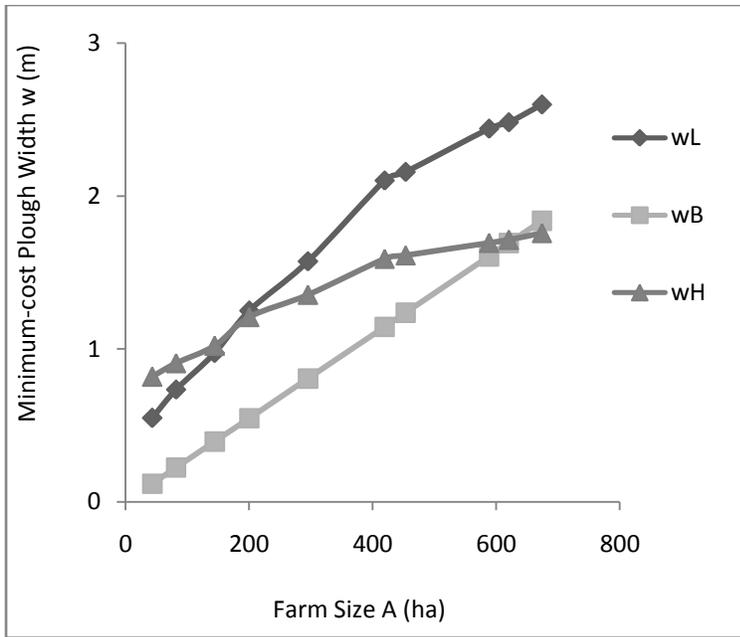
**Figure 2: Minimum-cost plough width for farm sizes variation**
