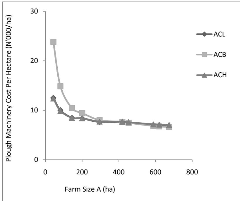
**Figure 3: Annual plough machinery cost per hectare for varying farm sizes**
