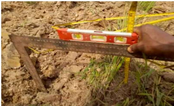
**Figure 1: Tillage depth measuring instrument**
