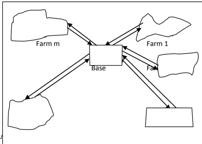
**Figure 1: Scattered pool m farms serviced from a single machinery base**
