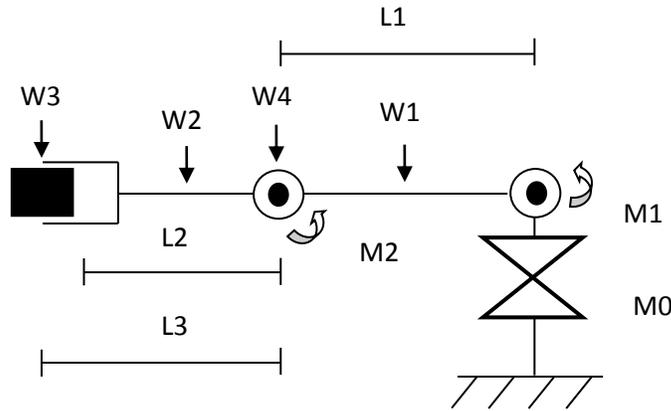
Figure 2: Force calculation of joints
