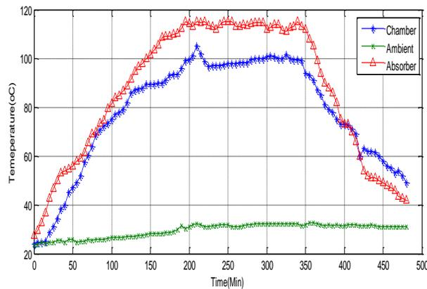
Fig.9: Temperatures during Stagnation Test on 31<sup>st</sup> March, 2016
