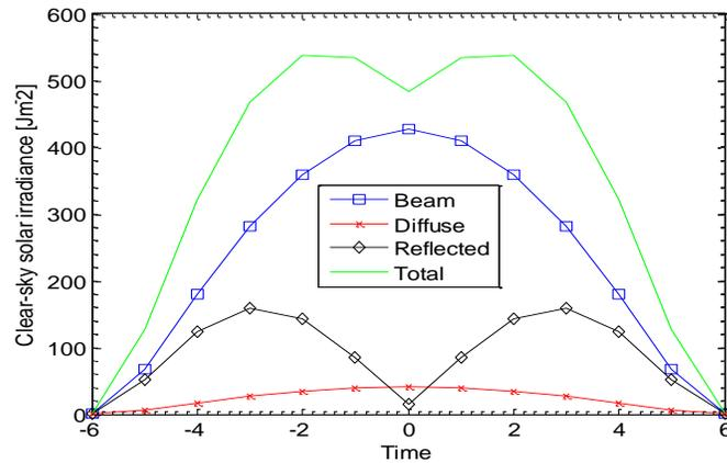
Fig.8. Clear-sky solar irradiance during sensible test on 1<sup>st</sup> April, 2016
