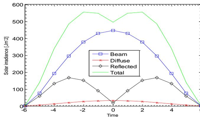
**Fig.7. Clear-sky solar Irradiance during stagnation test on 31<sup>st</sup> March, 2016**
