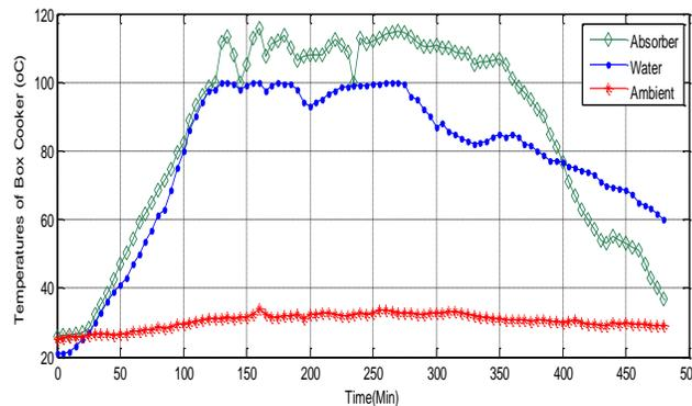
Fig.10: Temperatures during sensible test on 1<sup>st</sup> April, 2016
