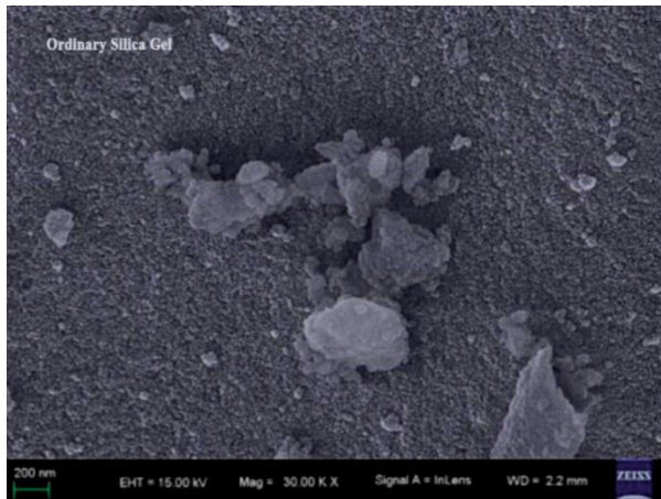
Figure 1a: SEM imagery of ordinary silica gel
