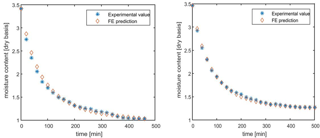
**Figure 9a & b. Measured moisture content and the FE predicted moisture content at heater temperatures of 120°C and 110°C for the Rectangular cassava sample**
