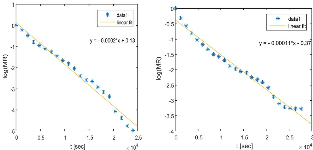
**Figure 2a & b. The plots of  $\ln(MR)$  against  $t$  for the Experiment at Heater Temperatures of 130°C and 120°C (70°C air temperature) (75°C air temperature) respectively for the rectangular samples**
