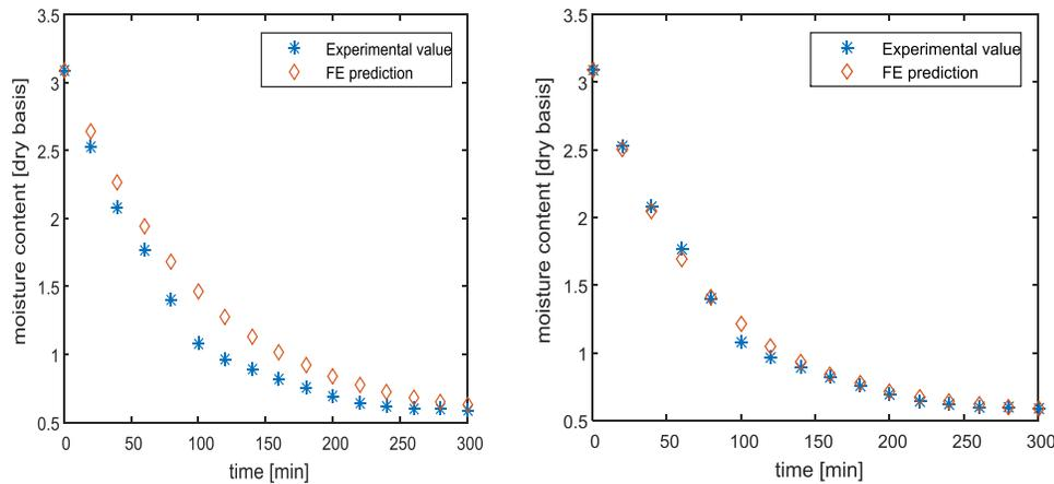
**Figure 7.** Measured moisture content and the FE predicted moisture content at heater temperature of 150°C for the Rectangular cassava sample (a) results for a (b) results for a 5447-elements model
