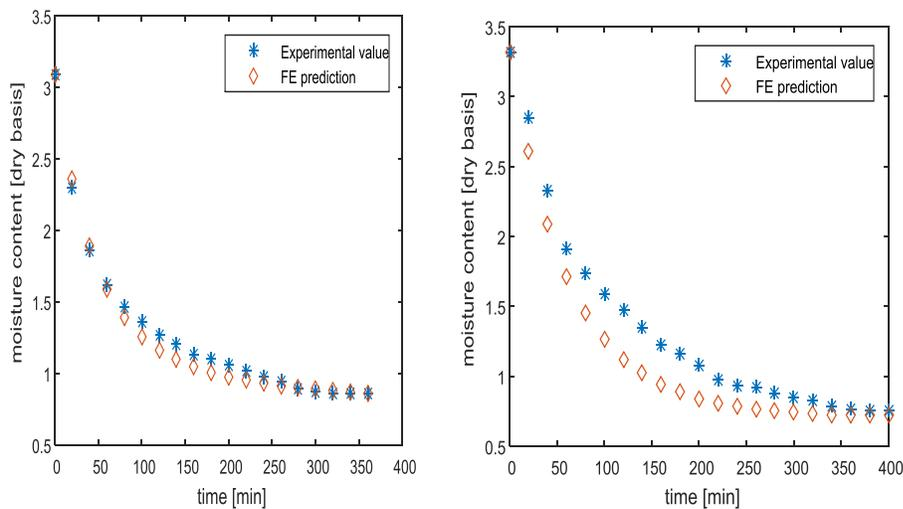
**Figure 8a & b.** Measured moisture content and the FE predicted moisture content at heater temperatures of 140°C and 130°C for the Rectangular cassava sample
