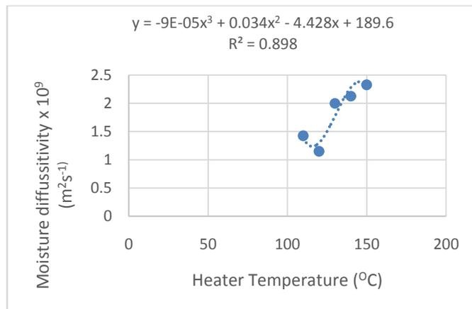
**Fig. 6:** Air temperature effect on effective moisture diffusivity for the Rectangular shape cassava pellets.
