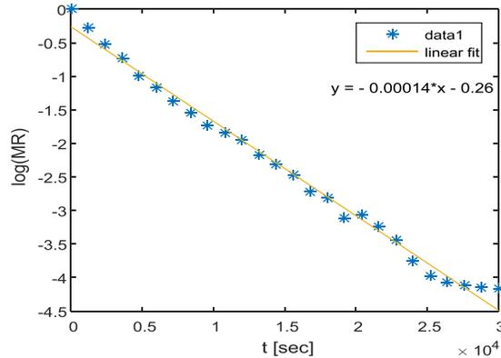
**Figure 3.** The plot of  $\ln(MR)$  against  $t$  for the Experiment at Heater Temperature of  $110^{\circ}\text{C}$  ( $66^{\circ}\text{C}$  air temperature) for the rectangular samples
