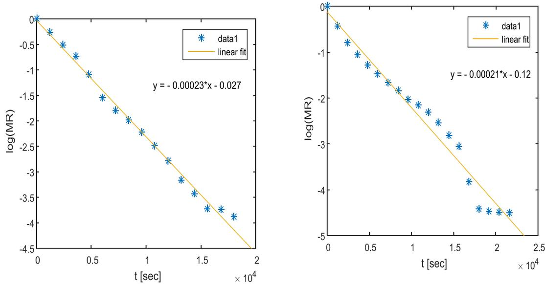
**Figure 1a & b. The plots of  $\ln(MR)$  against  $t$  for the Experiment at Heater Temperature of 150°C (81°C air temperature) and 140°C (78°C air temperature) respectively for the rectangular samples**
