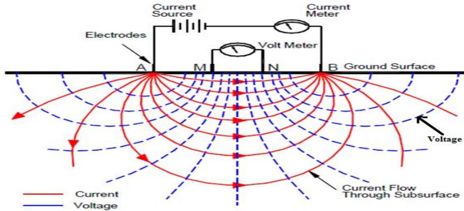
Figure 2: Schematic diagram Illustrating basic arrangement for Electrical Resistivity Measurement (Northwest Geophysical Associates, 2013).
