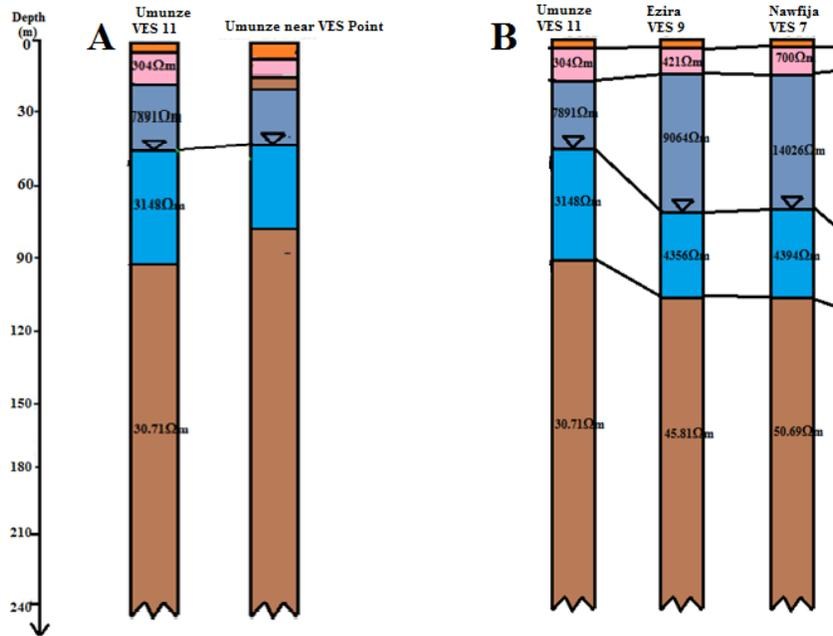
Figure 3: Geo-electrical section of some of the sample points
