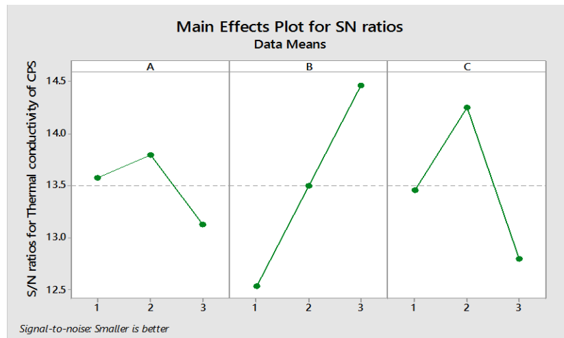
Figure 11: S/N ratio response graph for Thermal Conductivity of CPS hybrid fiber reinforced composite
