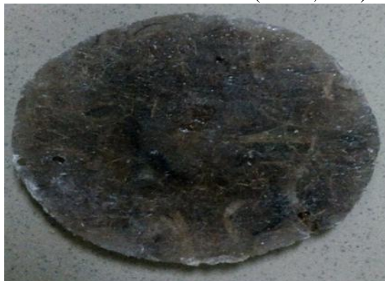
Figure 7: Thermal Conductivity Test specimen
