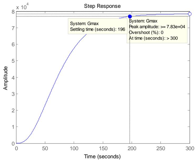
Figure 5: Step response of the heat exchanger model for the maximum parameters
