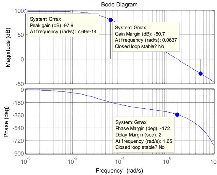
Figure 6: Bode plot for the maximum parameter value experiment
