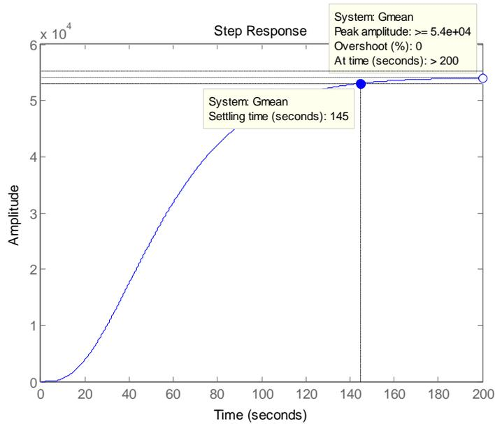
Figure 3: Step response of the heat exchanger model for the mean parameters
