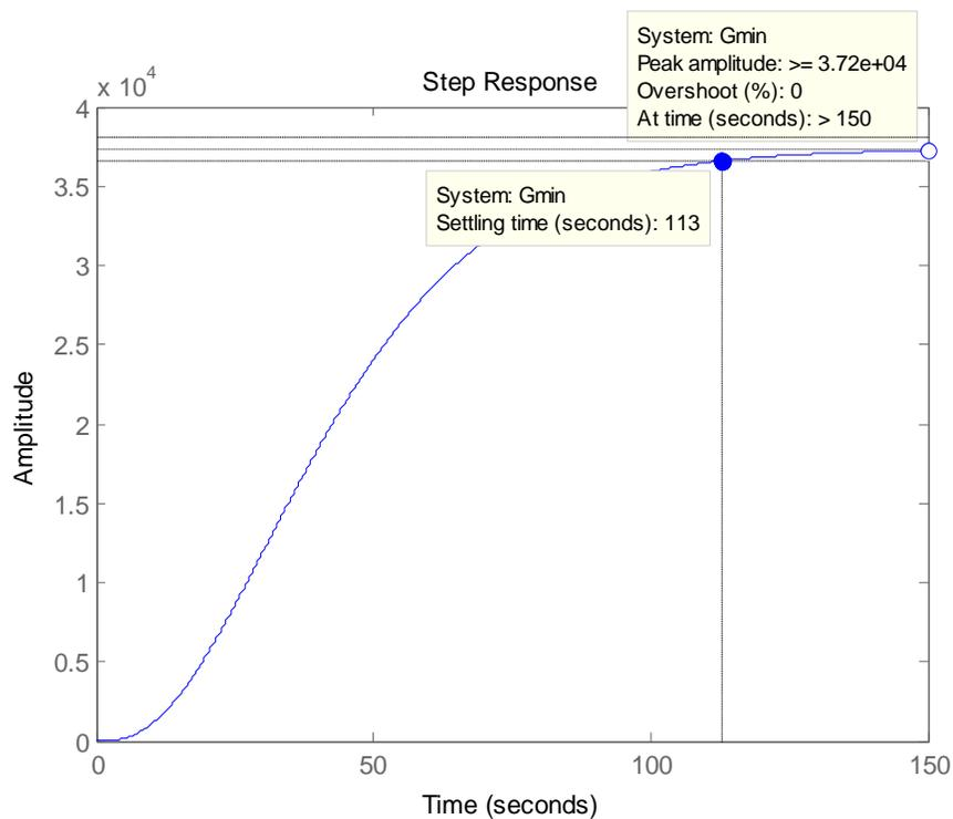
Figure 1: Step response of the heat exchanger for the minimum parameters
