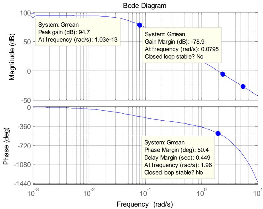
Figure 4: Bode plot for the mean parameter value experiment
