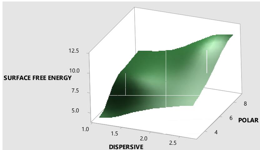
**Fig 11: 3D Surface Plot of Surface Free energy vs Polar and Dispersive Surface Free Energy for Epoxy**
