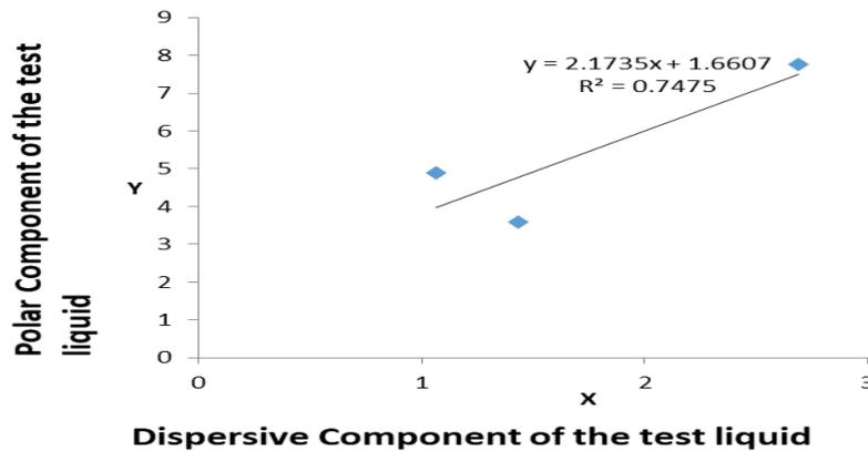
**Figure. 3: Scatter Plot of Fowkes Equation for Silicon Pressure Sensitive Adhesive to Derive Surface Free Energy for the Adhesive**
