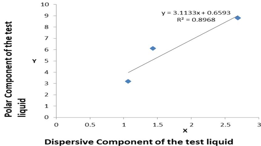
**Fig. 4: Scatter Plot of Fowkes Equation for Epoxy Pressure Sensitive Adhesive to Derive Surface Free Energy for the Adhesive**
