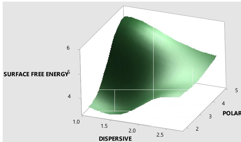
**Fig 10: 3D Surface Plot of Surface Free energy vs Polar and Dispersive Surface Free Energy for Mild Steel**
