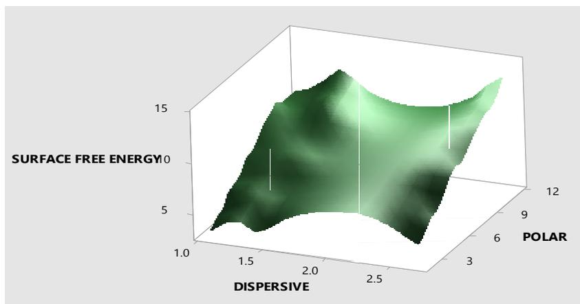
**Fig 7: 3D Surface Plot of Surface Free energy vs Polar and Dispersive Surface Free Energy for Cow Skin**
