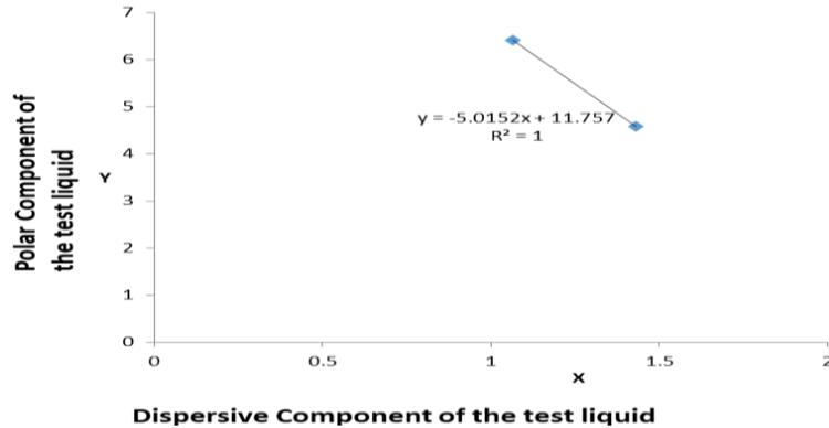
**Figure 2: Scatter Plot of Fowkes Equation for Acrylic Pressure Sensitive Adhesive to Derive Surface Free Energy for the Adhesive**
