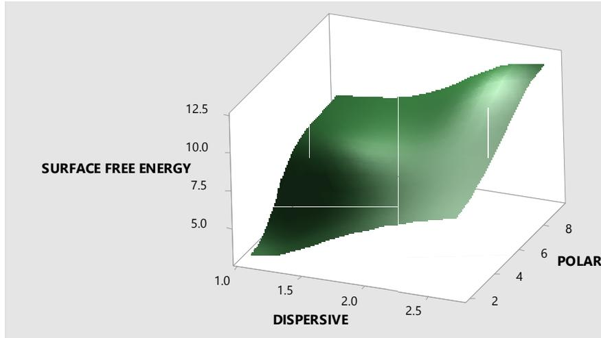
**Fig 9: 3D Surface Plot of Surface Free energy vs Polar and Dispersive Surface Free Energy for Natural Rubber**
