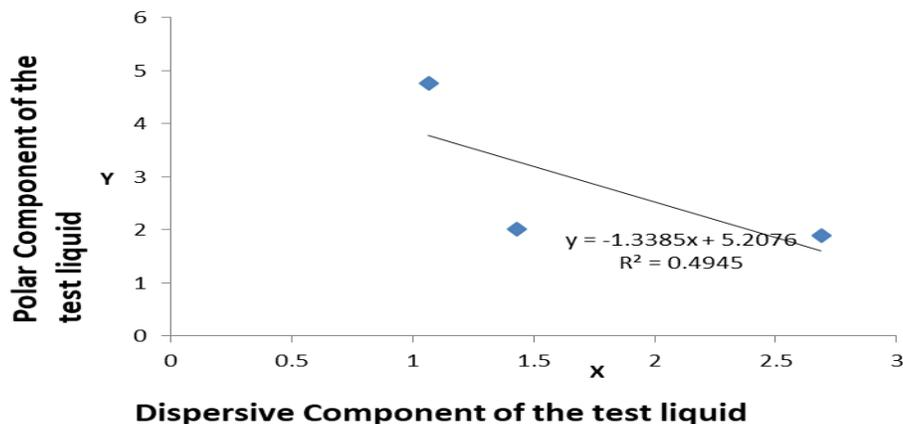
**Fig. 5: Scatter Plot of Fowkes Equation for Mild Steel Substrate to Derive Surface Free Energy for the Substrate**
