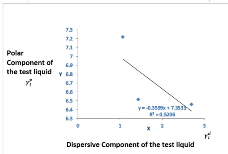
**Figure 1: Scatter Plot of Fowkes Equation for Cow Skin Pressure Sensitive Adhesive to Derive Surface Free Energy for the Adhesive**
