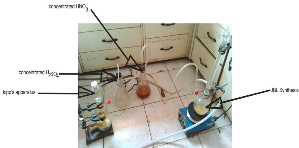
**Plate 2.1: Experimental setup for the Kipp's apparatus**
