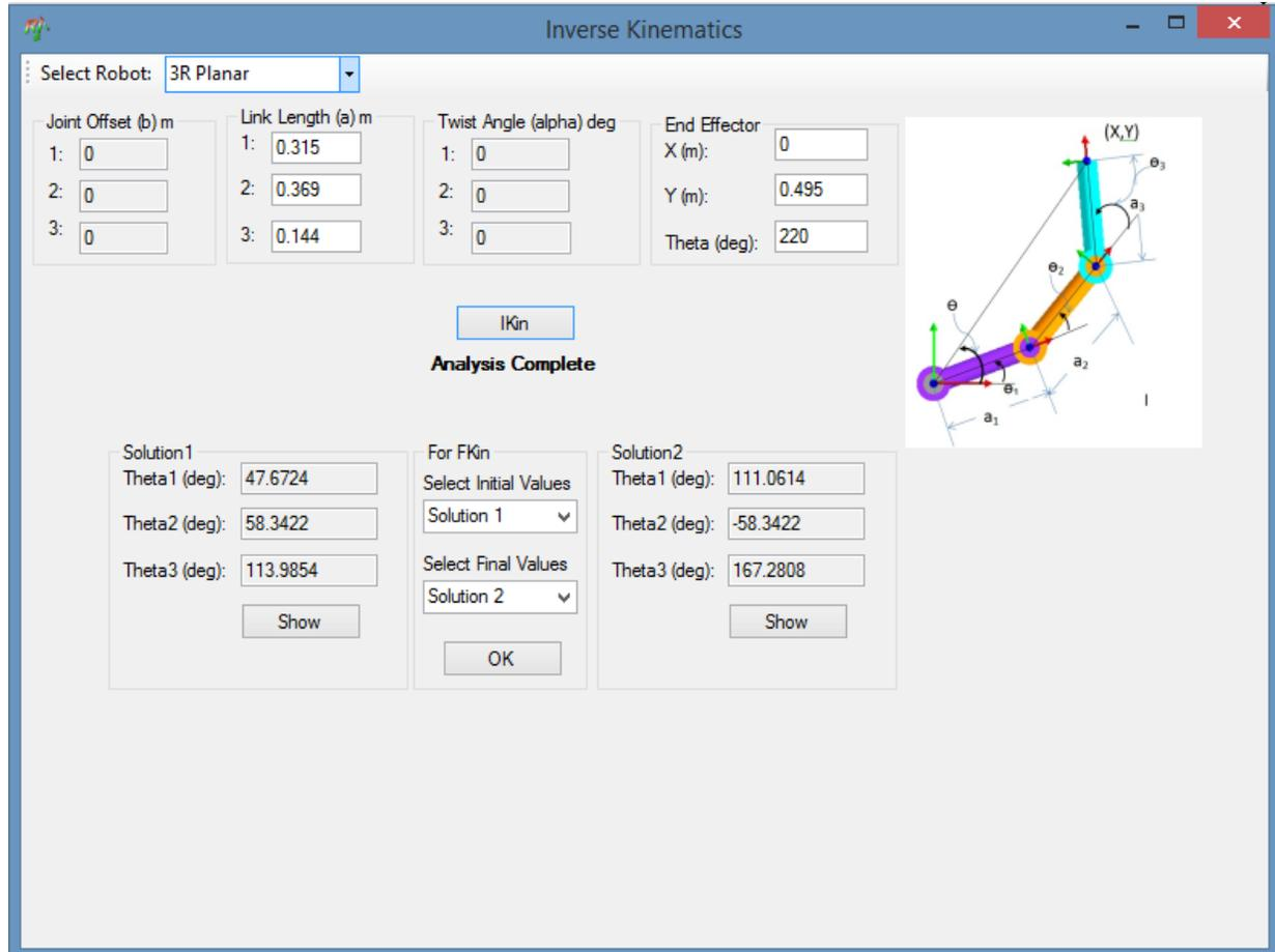
**Plate 1: Screen Snip of the RoboAnalyzer Inverse Kinematics Window Showing Results of the URL at P2**
