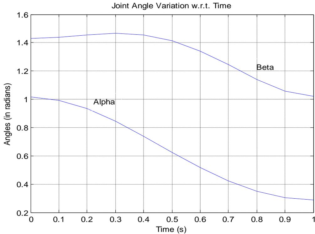
**Fig. 9: Joint Angles Variations of the LRL from P2 to P1**
