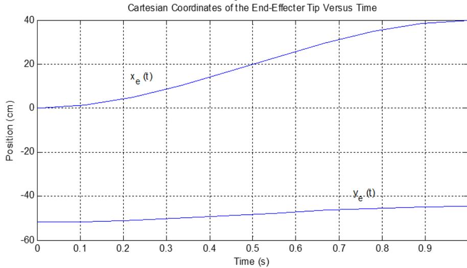
**Fig. 10: Position-Time History of the LRL's End-Effector Coordinates from P2 to P1**
