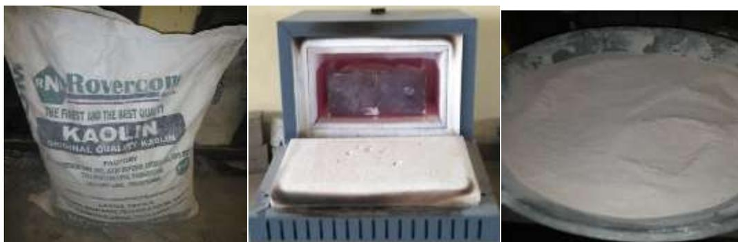
Figure 1: (a) Raw Kaolin Powder (b) Calcination of Kaolin in furnace (c) Metakaolin powder
