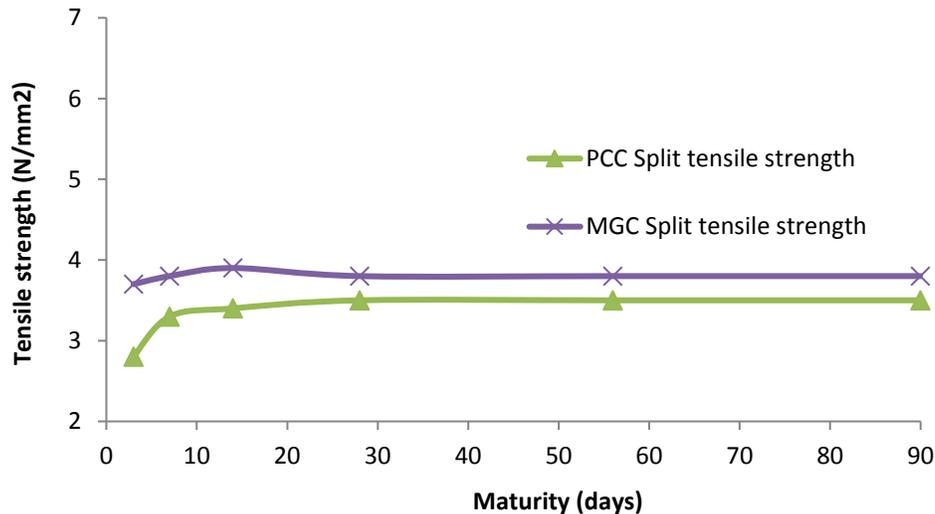
Figure 5: Split tensile strength of PCC and MGC
