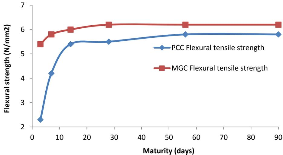
Figure 4: Flexural strength of PCC and MGC
