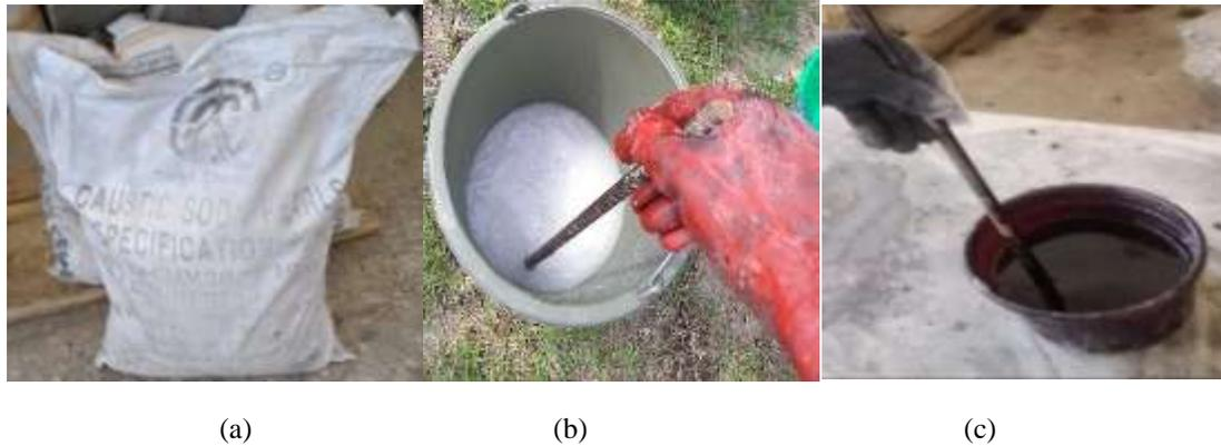
Figure 2: (a) Bag of sodium hydroxide flakes (b) Sodium hydroxide solution (c) Sodium silicate solution
