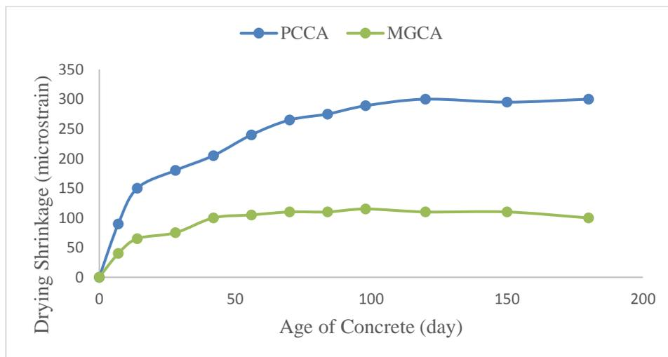
Figure 7: Drying shrinkage property of PCC and MGC
