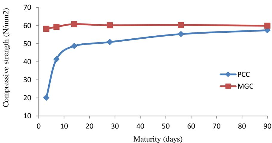
Figure 3: Compressive strength of PCC and MGC
