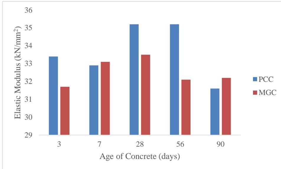
Figure 6: Elastic modulus of PCC and MGC
