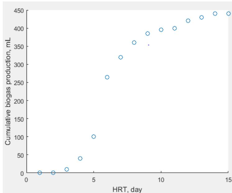
Fig. 12: Cumulative biogas production from modified Gompertz model of YMP digestion
