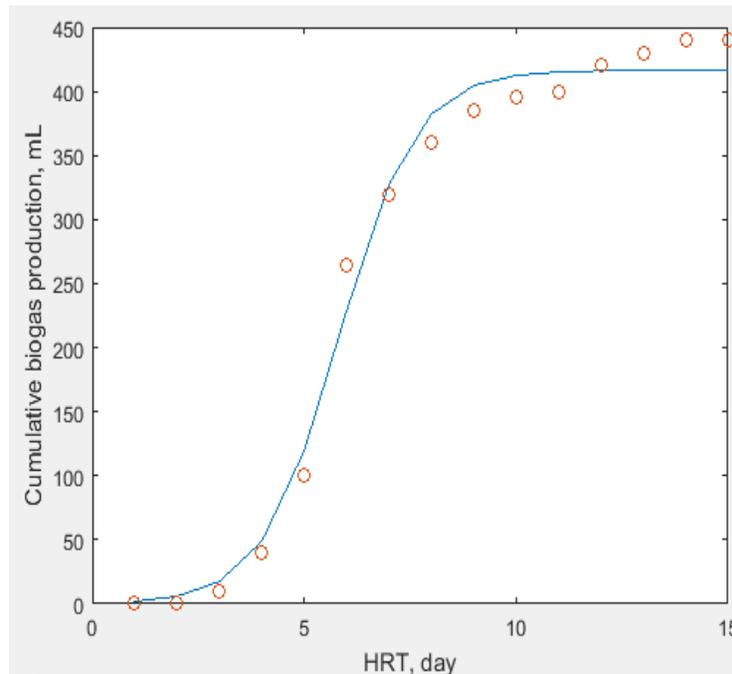
Fig. 11: Cumulative biogas production from modified logistic model of YMP digestion
