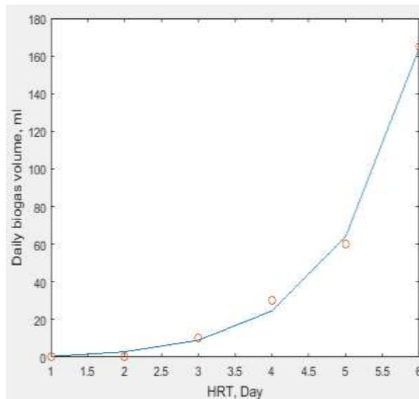
Fig. 6: Biogas production rate from exponential model (ascending limb) of YMP digestion
