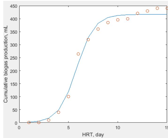
Fig. 10: Cumulative biogas production from logistic model of YMP digestion
