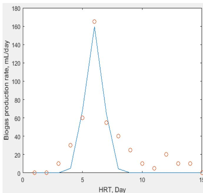
Fig. 8: Biogas production rate from Gaussian model of YMP digestion
