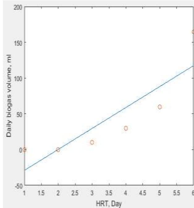
Fig. 4: Biogas production rate from linear model (ascending limb) of YMP digestion
