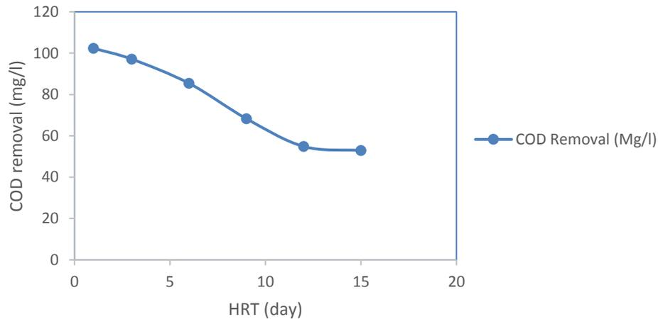
Fig. 1: COD removal with HRT on YMP digestion
