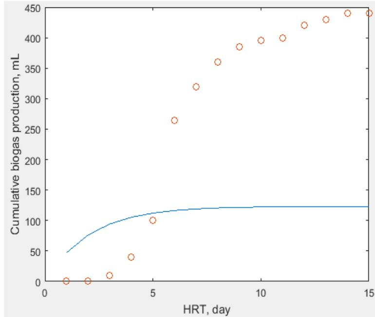
Fig. 9: Cumulative biogas production from exponential rise to maxima model of YMP digestion
