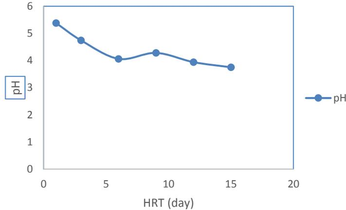
Fig. 3: Variation of pH with HRT on YMP digestion
