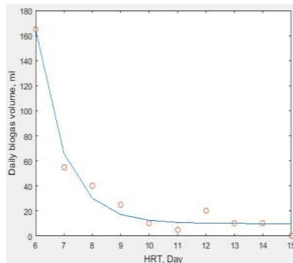
Fig. 7: Biogas production rate from exponential model (descending limb) of YMP digestion
