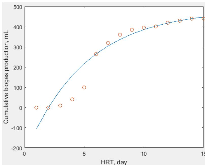
Figure 13: Cumulative biogas production from transference model of YMP digestion
