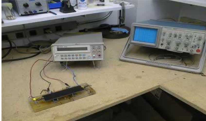
Figure 2 Circuit set up for Ohm's experiment
