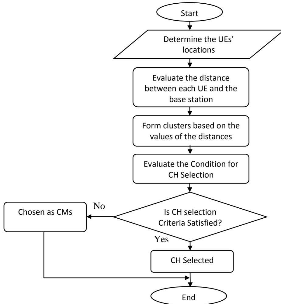
Figure 3: Flow Chart Showing the Cluster Formation Procedure
