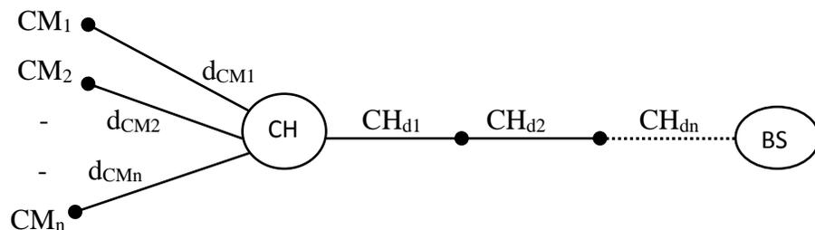
Figure 2: Factors Influencing Energy Consumption of Cluster Head (CH)
