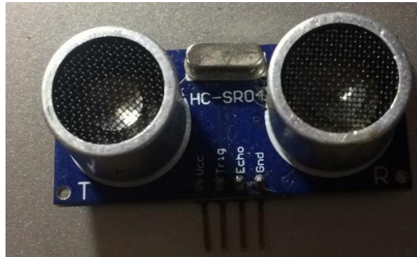
Figure 2 HC-SR04 ultrasonic proximity sensor
