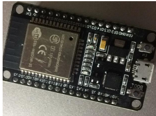
Figure 3 Wifi enabled Esp32 WROOM-32 microprocessor
