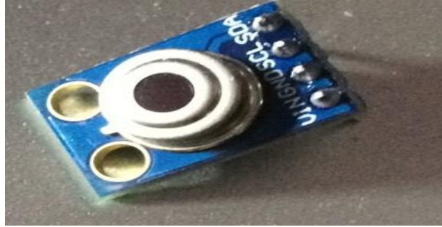
Figure 1 By-906 Infrared Arduino Temperature Sensor
